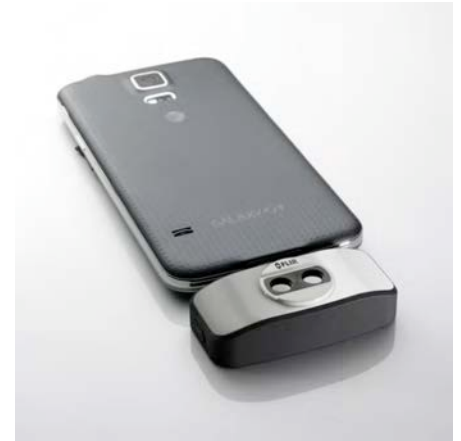
Figure 27.3 2015: FLIR One, an accessory to iPhone and Android mobile phones. Weight: 90 g (3.2 oz.).
